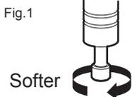
Turn loosen the adjustable knob counter-clockwise to the end before placing the steering damper body in place.
