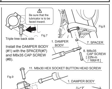
12. M8 NUT Have the BODY CLAMP (#10) and slide it onto the STEERING DAMPER BODY(#1). Attach the BODY CLAMP(#10) onto the FRAME BRACKET(#2) as per the picture.
