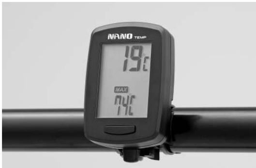
The following temp. gauge and fitting are available from Daytona. The temp. gauge (#85995) can be used with the Daytona oil cooler (#74019) by using the Daytona sensor fitting (#43350).
